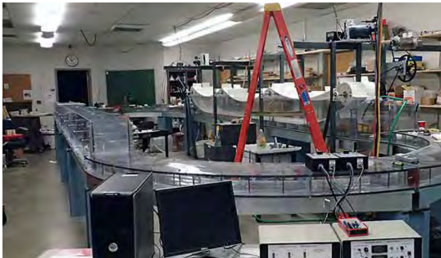
The wave and tide flume in the 5th floor flume lab. It is a unique facility with sophisticated electronic controls that allow us to program entire experiments so that they can be repeated identically as specific variables are modified to explore parameter space.
